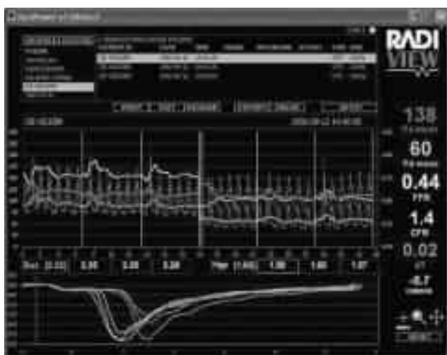
Figure 13-20 Example of simultaneous pressure and temperature tracings. The top tracings represent central aortic pressure (Pa) and distal coronary pressure (Pd), and FFR (Pd/Pa). The lower tracings are temperature tracings recorded by the proximal (shaft) and distal sensors. The half-time of injection was derived from the proximal thermodilution curve. Coronary flow volume is calculated from the distal thermodilution. Tmn at hyperemia, \text{CFR} = \text{V/Tmn at hyperemia} , \text{V/Tmn at rest} \text{CFR} = \text{Tmn at rest} . (Courtesy of St. Jude Medical, Minneapolis, MN (Figure formerly provided by Radi Medical, Uppsala Sweden), Uppsala, Sweden.)
