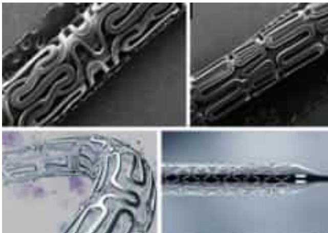
Figure 7-9 Cell designs of drug-eluting stents: Cypher (top left), Taxus (top right), Xience (bottom left), Endeavor stent (bottom right).
