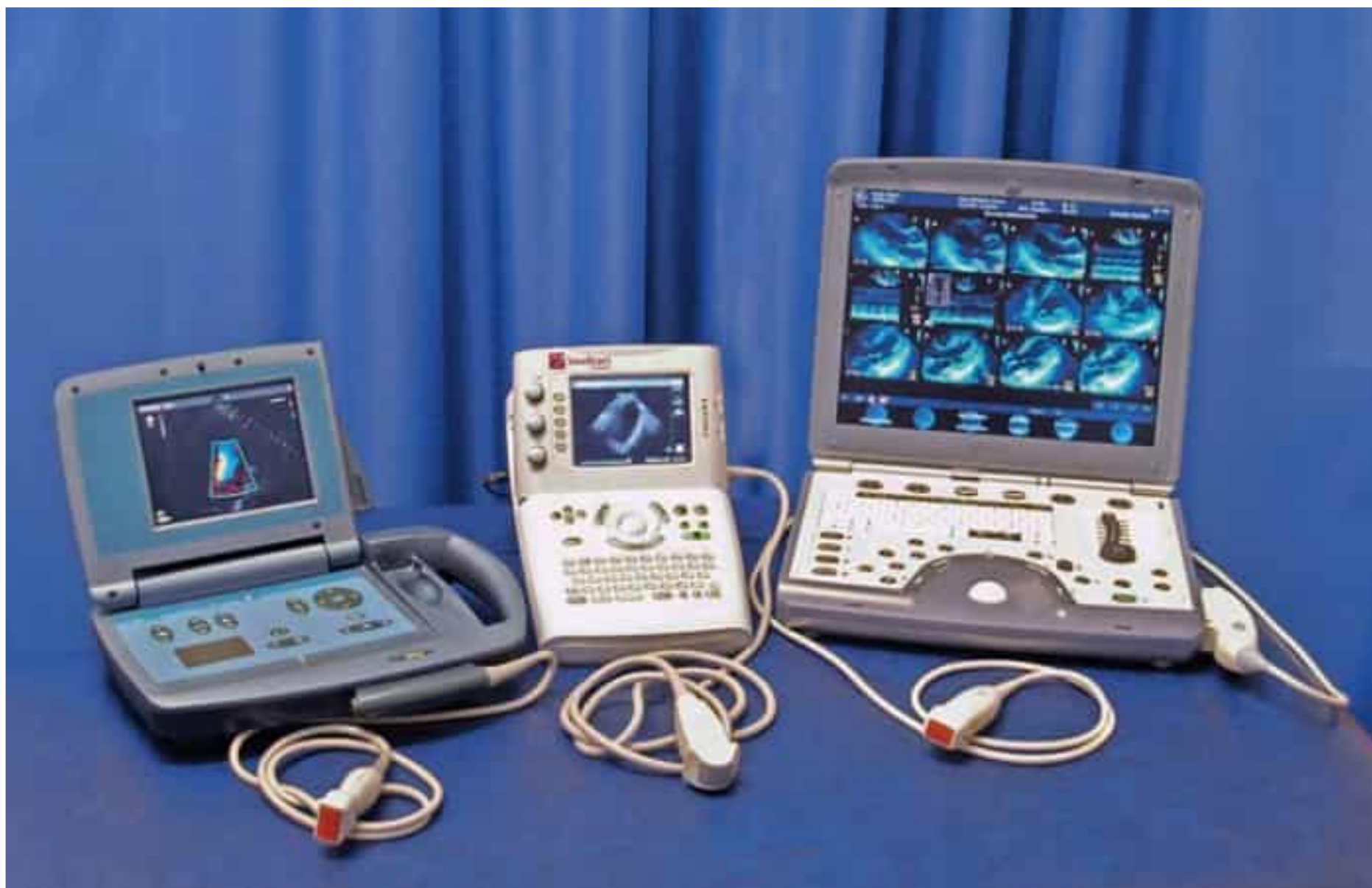
Fig. 2.4 Miniaturized ultrasound systems for bedside or ambulatory imaging (Optigo, Philips Sonoline, ViVid I GE).
