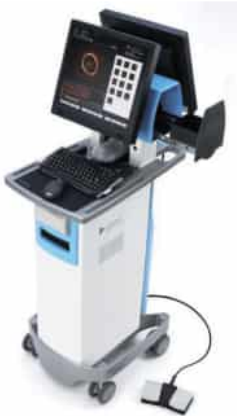
Figure 11.1. The mobile OCT cart incorporating the system console, monitor, and patient interface unit.
